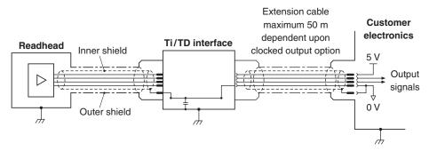
**IMPORTANT:** The outer shield should be connected to the machine earth (Field Ground). The inner shield should be connected to 0 V at receiving electronics only. Care should be taken to ensure that the inner and outer shields are insulated from each other. If the inner and outer shields are connected together, this will cause a short between 0 V and earth, which could cause electrical noise issues.
