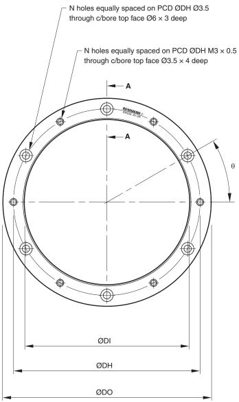
**NOTE:**  $\theta$  is the angle between one tapped hole and the adjacent clearance hole. The angle between two clearance holes is  $2\theta$ .
