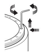
**NOTE:** At this stage, the screws should only be lightly tightened (less than 0.5 Nm) to allow further final adjustment.
