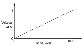
Set-up signal voltage proportional to incremental signal amplitude
