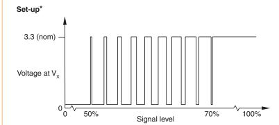
Between 50% and 70% signal level,  $V_{\chi}$  is a duty cycle.
