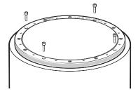
Insert screws into the remaining mounting holes.
