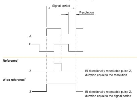
**NOTE:** Select 'standard' or 'wide' reference at time of ordering, to match the requirements of the controller being used. Wide reference mark not available on Ti0004 interfaces.
