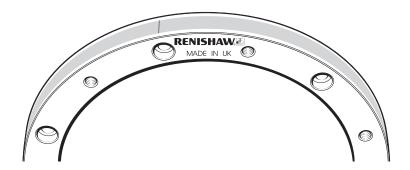
*IN-TRAC*™ reference mark is integrated in the scale, radially aligned with the centre of the mounting hole to the left of the 'Renishaw' logo within ±0.5 mm.
