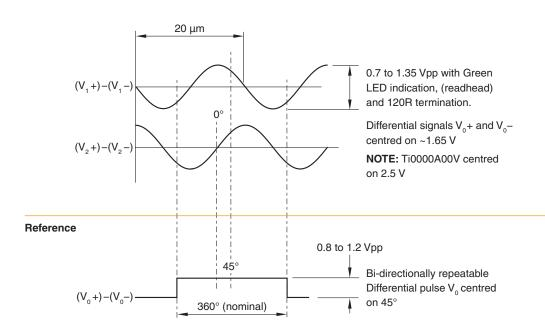
Limits Open collector output, asynchronous pulse
