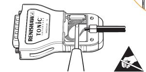
▶ Refit the cover plate ensuring the cable ferrule is located in the recess on the inside and no wires are trapped under the cover plate.
