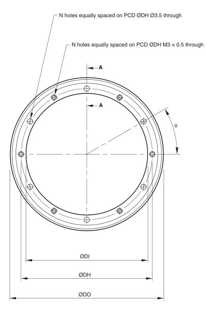
**NOTE:**  $\theta$  is the angle between one tapped hole and the adjacent clearance hole. The angle between two clearance holes is  $2\theta$ .
