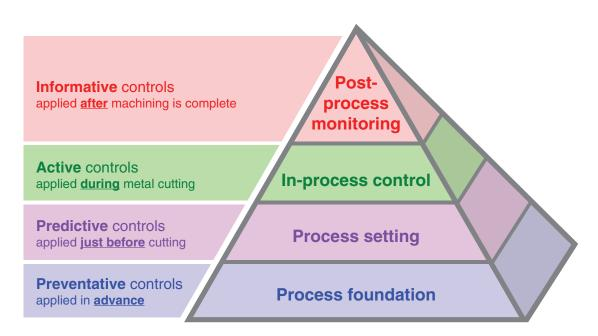
Figure 1: Renishaw's Productive Process Pyramid™
