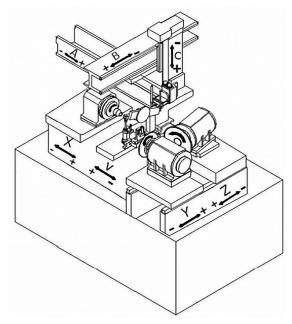
Schematic of TGT's Microma Auto grinding machine
