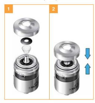
6. Reassemble the stylus to the probe as shown below.
