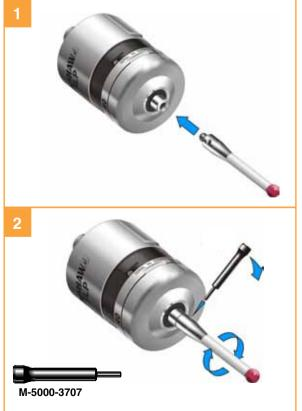
7. Check stylus on-centre and adjust if necessary.
